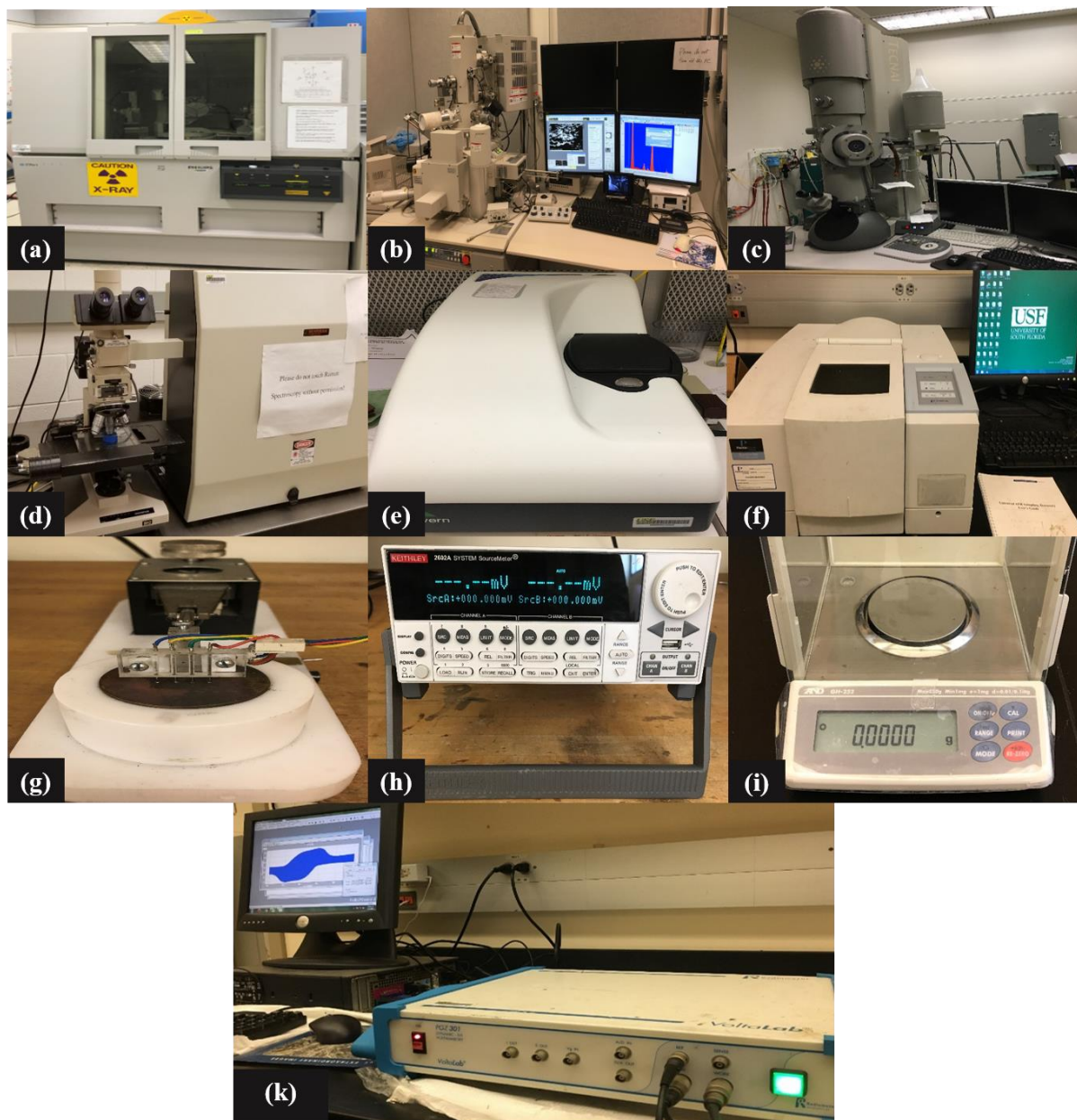
Figure 3.1 Instruments were used for all the characterizations (a) XRD, (b) SEM, (c) TEM, (d) Raman spectroscopy, (e) PSA, (f) FTIR, (g) four-in-line probe setup, (h) Keithley source meter, (i) analytical balance and (j) Radiometer Analytical Voltalab 40.
